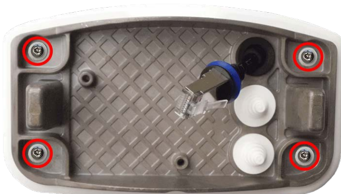
Fig. 6: Installed and ready for Connector Box RJ45
