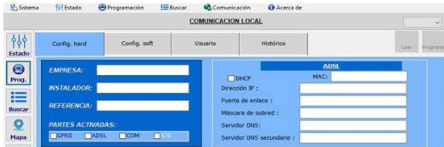
All parameters are read automatically, when we modify a parameter it will appear red, to indicate that it has been modified and that it is pending being sent to the circuit.
