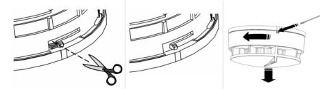
If you want to extract a detector that has been locked, it is necessary to insert a screwdriver into the slot to release the locking tab, rotating the detector anti-clockwise at the same time
