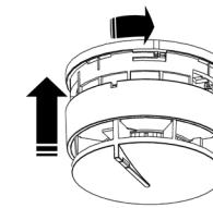
The detectors have a locking system to help prevent unauthorised detector removal. As supplied, the detectors can be removed without use of an extraction tool (useful for high ceilings).
