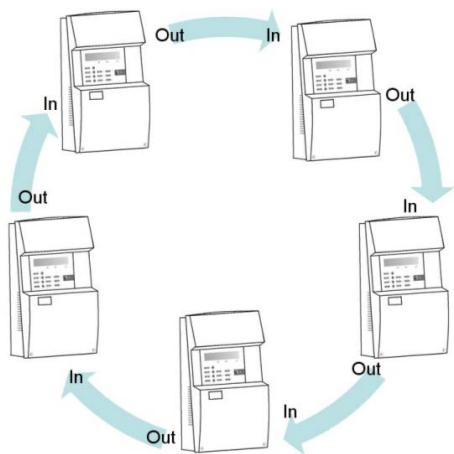
TMB-251-LT card includes 2 RS485 serial ports for input and output S-Network connection. Set the JP3 jumper position for addressable panel mode. Connect the terminals from the connectors RS485 indicated as OUT (B, A y  $\pm$ ) to the corresponding ones of the RS485 connected indicated as IN (B, A y  $\pm$ ) in the next equipment (a control panel or another repeater). So on until returning to the repeater.
